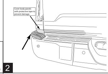
Remove license plate light by rotating and pulling out. Squeeze metal tabs holding trailer hitch plug and remove.
