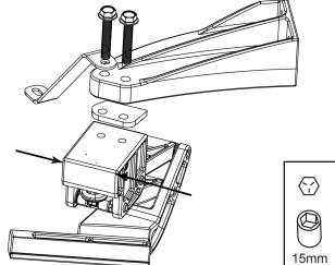
Remove corner bumper cap and use flat blade screwdriver to pry loose. Use caution when removing tabs.
