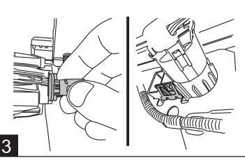
Remove plastic plug holding bumper cap onto lower portion of bumper. Remove license plate and plug behind holding bumper cap in place.
